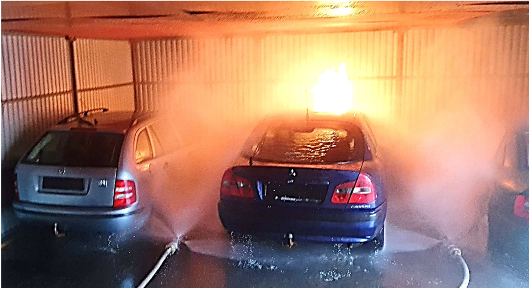
Figure 5 Boundary Cooling Device in operation (Handling Tests)
