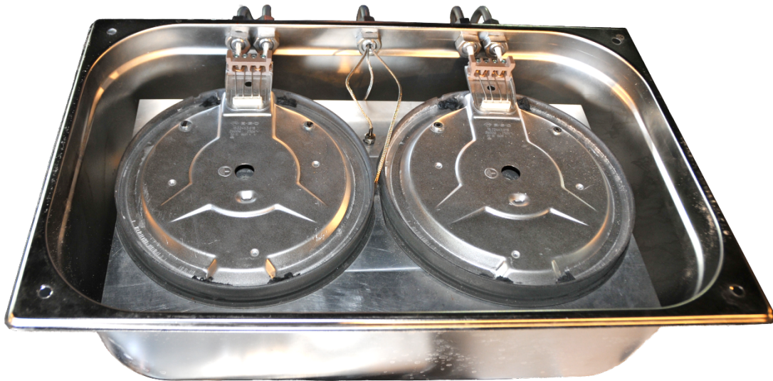
Figure 2: View Inside the Open Battery / Gas Tank Dummy
