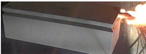
Figure 2: Prepared bicycle battery at the moment of ignition during thermal runaway
