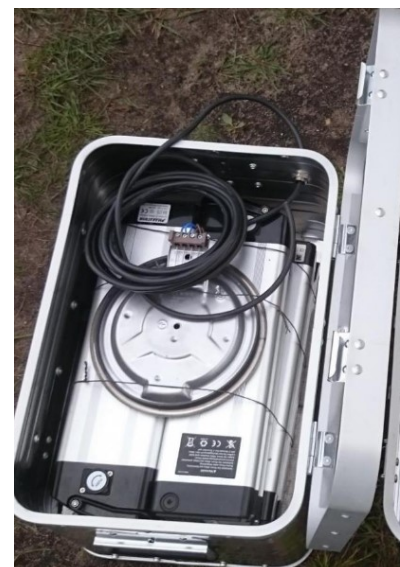
Figure 3: Setup: 4 batteries in a box, hotplate as ignition source
